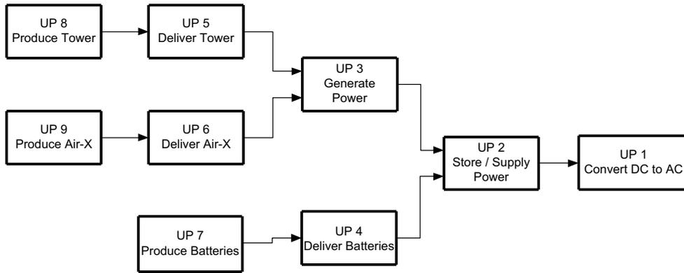
Fig. 1. Process flow diagram for all unit processes of the wind system that are within the boundary of the study.
